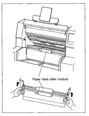
**4** Draw the paper feed roller module toward you and remove it starting with its left side.
